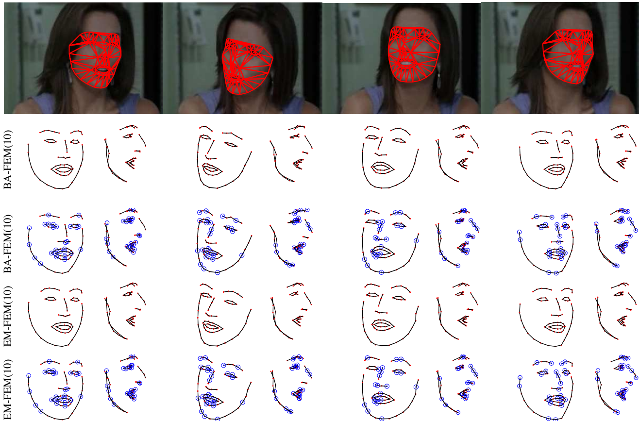
Fig. 14 Actress sequence. Selected frames #31, #48, #84 and #102. First row: Image frame sequence with 3D reprojected mesh. Second and third rows: Original viewpoint and side views of the 3D reconstruction in the cases of full data and 40% missing data, respectively, using the BA-FEM algorithm. Fourth and fifth row: The same views applying the EM-FEM algorithm in the cases of full data and 40% missing data, respectively. Visible points are displayed in red dots, and occluded points in blue circles.
