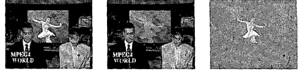
Figure 6. Example of motion connected operator preserving still objects: original frame (left), operator (center), residue (right).
