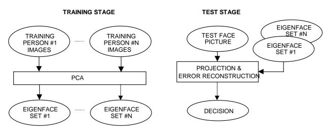
Figure 1. Block diagram of the self-eigen approach for face recognition
