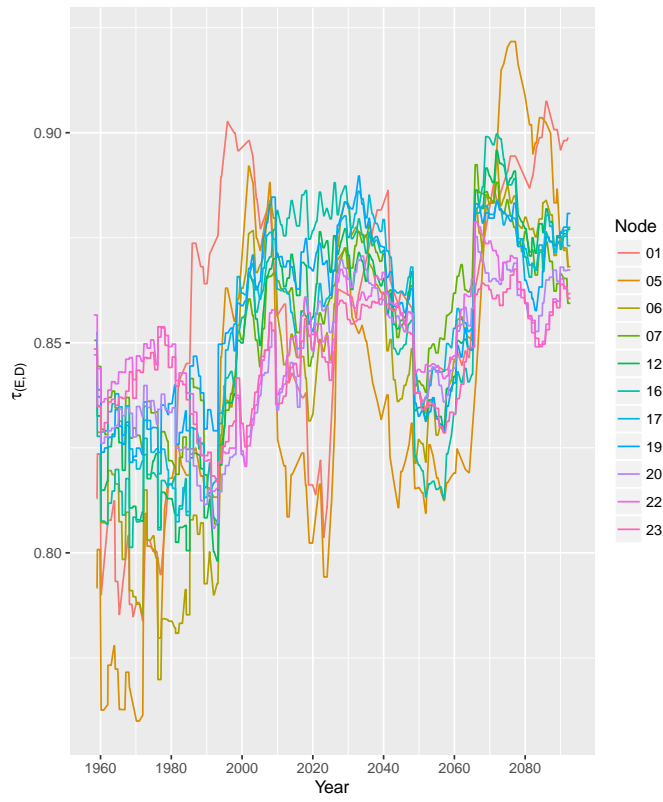
Figure 10: Non-stationary \tau_{(E,D)} dependence parameter at the (E,D) nesting level of the HAC. The marginal distributions are fitted with the VGAM, with time as the sole covariate (NS-T).
