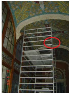
Figure 5 - In-situ dynamic identification test: (a) location of the accelerometers in the tested vaults, (b) positioning of the experimental set up in vault A and (c) accelerometer used for measurements of vault A.
