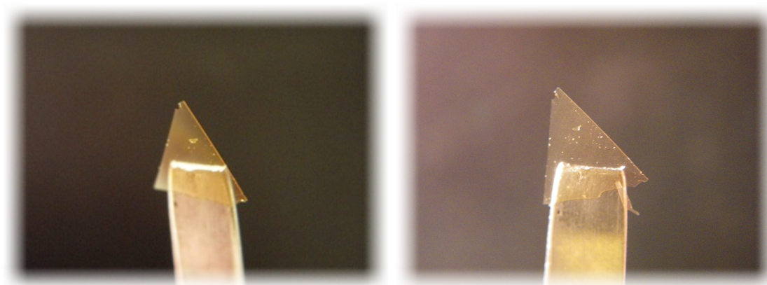
Figure 5.24: Photographs of a sample of polymer film cut from the film formed on the petri dish. Film placed on end of a spatula for size reference.
