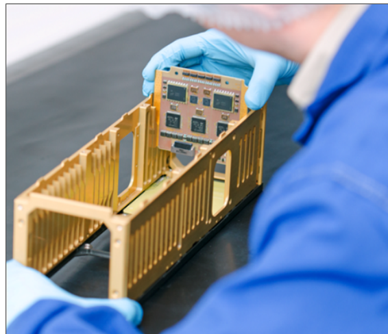
Figure 4: C3S 3U CubeSat Structure. Image courtesy of Complex Systems and Small Satellites (2015).
