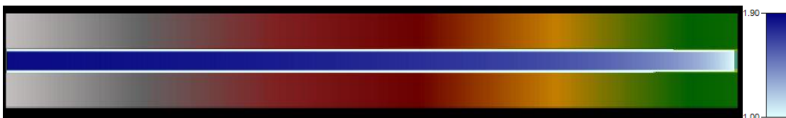
Figure 5.1.5.4. Water depth in the case of M2 curve in the channel. Units in metres.
