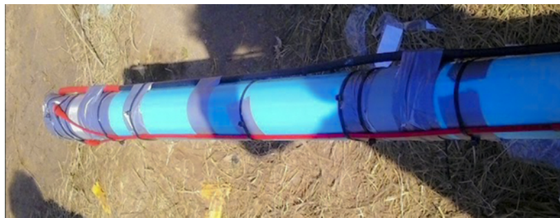
(c) PVC tube with optical fiber (in red)
