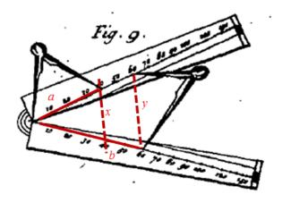
Figure 1. General use of the sector, in Stone (1723), plate VII, Fig. 9 [digitized by the Internet Archive, 2012, with funding from Gordon Bell, available at <a href="http://archive.org/details/constructionprin00bion">http://archive.org/details/constructionprin00bion</a>]. Red lines added by the author.
