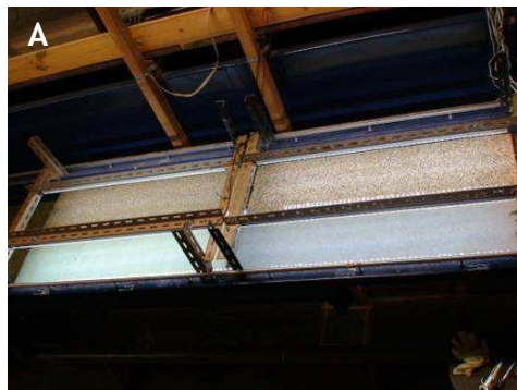
Figure 3. 6. Growth characteristics of the central box of the rows. As it is visible from the image, due to the different flow patterns in the centre of the box (see arrow) not subjected to wall effects, the growth was different from the other boxes. Hence the decision of testing only the boxes directly in contact with the walls (e.g. box 1 and box 3).
