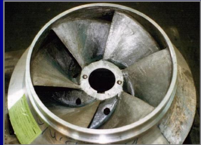
“AS SUPPLIED” ROUGH VANE SURFACE
