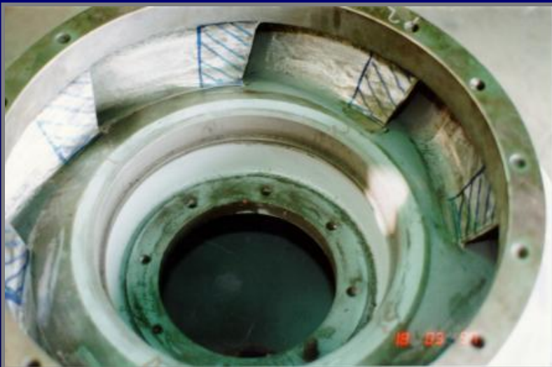
VANE CUT MARKING
