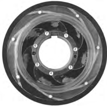
Figure 12. Varnish Damages in Impeller #1 at Q = 0.049 \text{ m}^3/\text{s} , N = 3000 \text{ RPM} , \Delta h = 7.8 \text{ m} .
