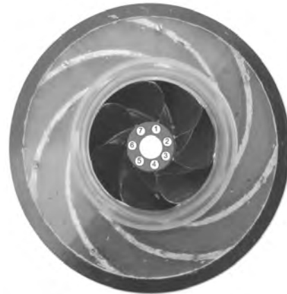
Figure 15. Centrifugal Impeller #2 after Tests at Q = 0.049 \text{ m}^3/\text{s} , N = 3000 \text{ RPM} , \Delta h = 7.8 \text{ m} .
