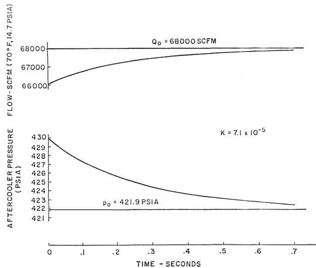
Figure 4. Transition Between Two Stable Operating Points.
