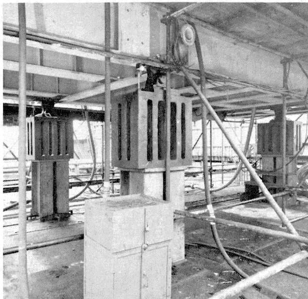
Figure 2. Three-Point Skid Support on the Test Stand.
