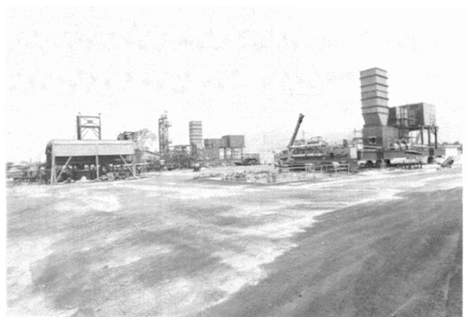
Figure 12. Massa 1982 — Outdoor Test Facilities with Two Stands — Preparation of a Single-Lift Module for Testing.
