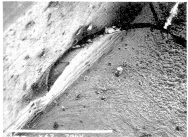
Figure 34. SEM Fractograph of the Dynamometer Wheel in Figure 33 Showing Cavitation Pitting Nucleation for Fatigue Failure of the Blading.
