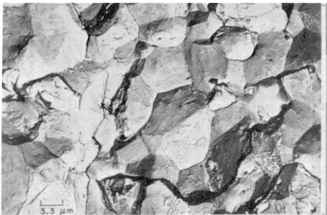
Figure 25. TEM Fractograph of an Intergranular Failure from Stress Corrosion Cracking.
