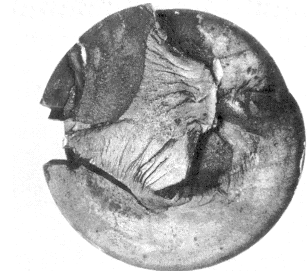
Figure 10. Combination Torsional and Bending Fatigue Failure of a Zirconium Alloy 705 Pump Shaft Due to a Loose Impeller.
