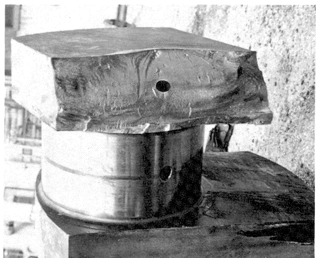
Figure 5. Failure of a Large 12 Inch Diameter Journal Reciprocating Engine/Compressor Crankshaft. The failure mode was fatigue in bending caused by main bearing misalignment.
