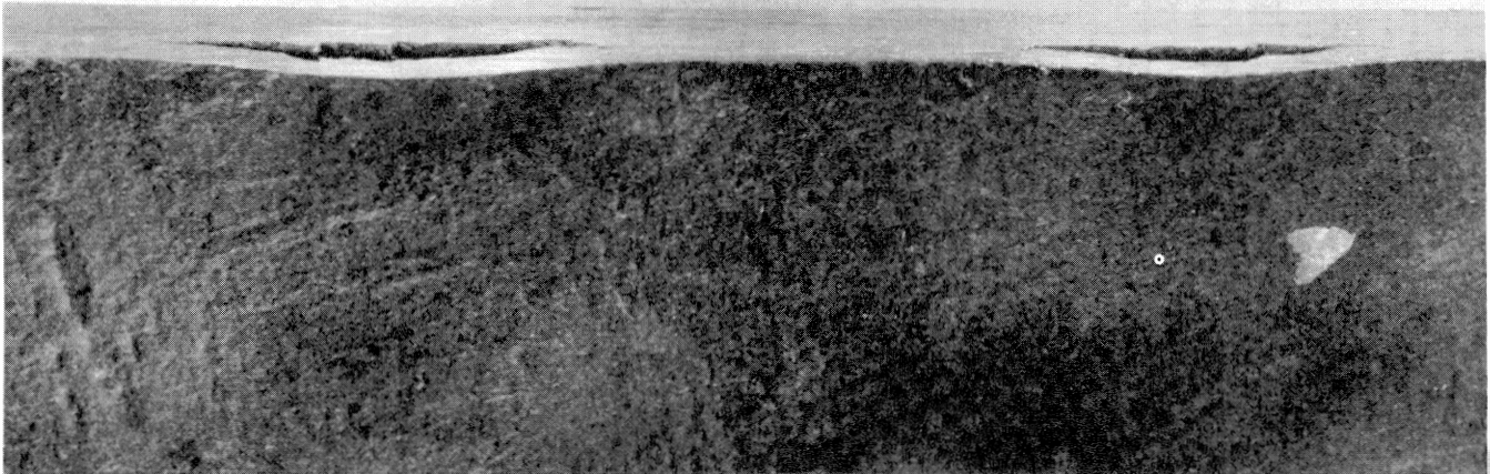
Figure 27. Cross Section of Plate in Figure 26 through Blisters Showing Delamination of Plate at Defects from Hydrogen Diffusion Combining to Molecular Form and Expanding.
