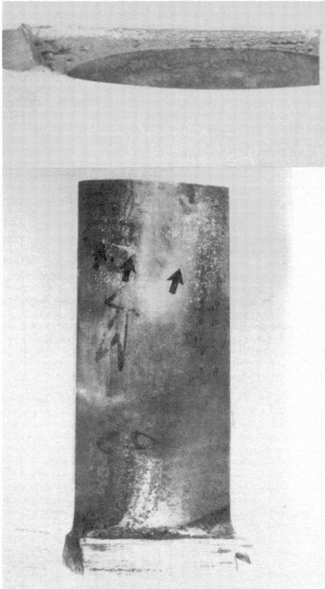
Figure 17. Crack in a Compressor Turbine Blade Which Was Identified as Having Failed by High Cycle Fatigue. The surface has the typical smooth appearance of a fatigue crack.
