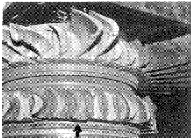
Figure 1. Blade Root Section (Identified by the Arrow) Chosen for Analysis Due to Its Discoloration. This blade was found to have failed in creep, causing the remainder of the damage.
