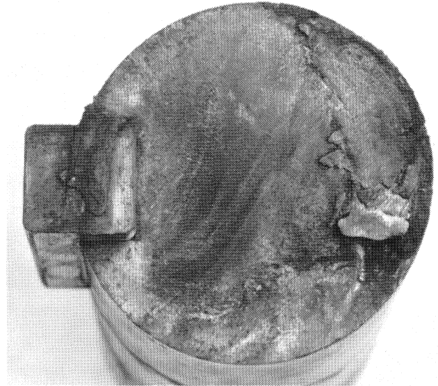
Figure 12. Bending Fatigue Failure of a Pinion Gear Shaft Due to Improper Alignment.
