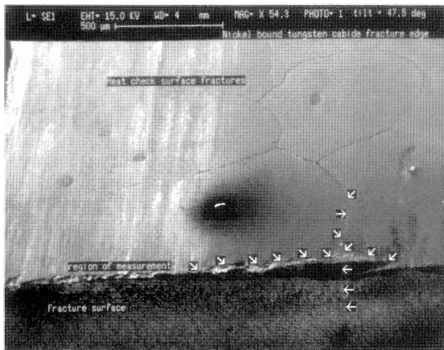
Photograph displaying surface fractures (heat checks) adjacent to the fracture surface
