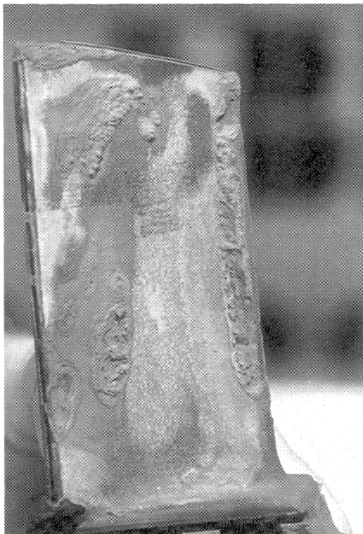
Figure 42. Hot Corrosion Damage.
