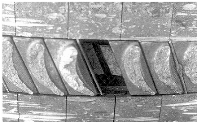
Figure 74. Blade Breakage at Root through Cooling Hole.
