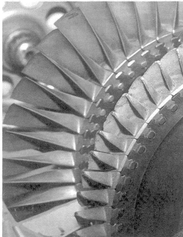
Figure 19. Burnt Blading Due to Fire in Turbine Section (Fuel Accumulation in Combustors).
