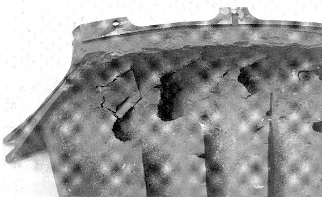
Figure 48. Typical Parabolic Trajectory Caused by an FOD/DOD Failure.
