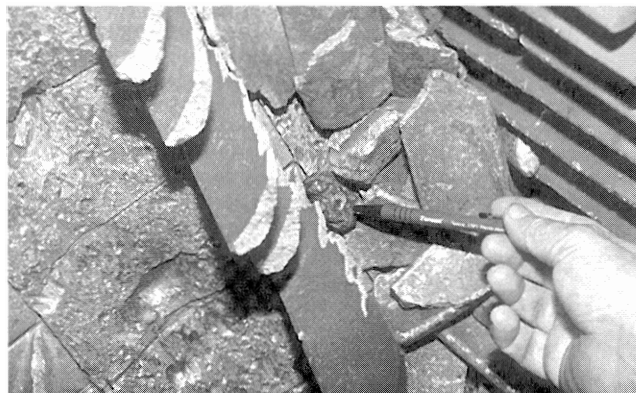
Figure 75. Battered Pin Found in Turbine Debris (Lower Turbine Casing). (This indicates the importance of a careful search of the debris. Missing this evidence on a similar failure in the past, resulted in this "repeat" failure.)
