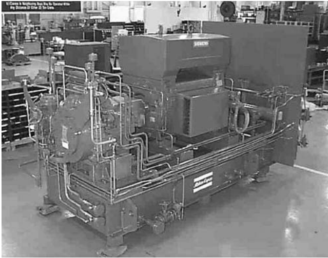
Figure 4. Oxygen Compressor, Integally Geared Design.
