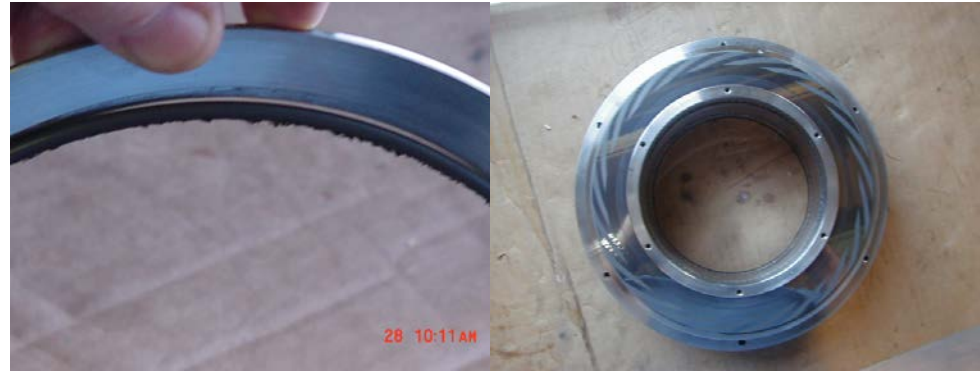
Primary Seal O-Ring and Tungsten Face – As removed from Compressor
