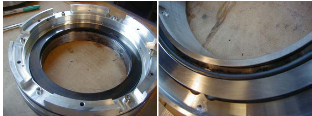
Secondary Seal – As removed from Compressor
