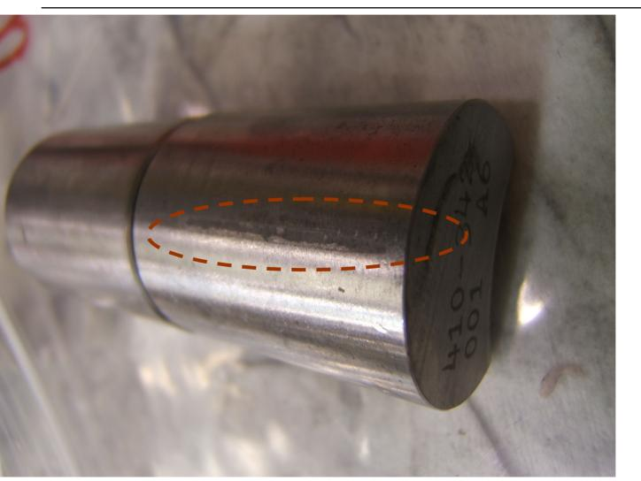
Flattened portion of the back of one of the loaded pad on the bearings of the third stage
