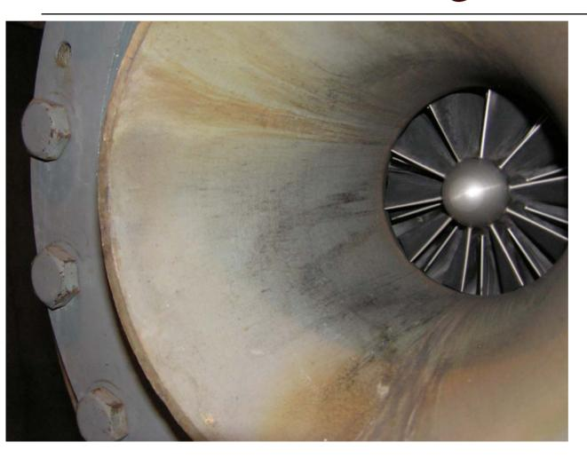
Inlet cone of the 2<sup>nd</sup> stage. Picture shows normal wear. The first intercooler and inlet piping showed only normal wear as well
