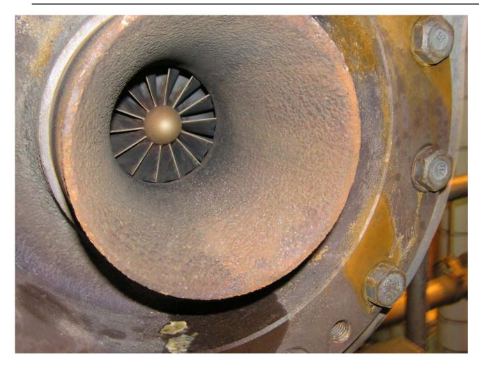
Inlet cone of the third stage. Picture shows heavy rust on the cone and deposits on the impeller. The inlet pipe was corroded beyond repair.
