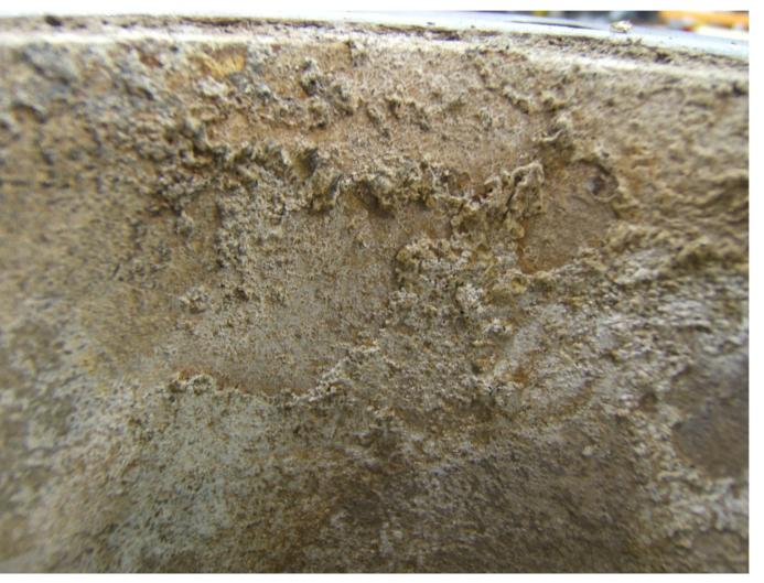
Scales found in the 3<sup>rd</sup> stage discharge horn. Seems to be the same kind of material deposit as found in the volute.
