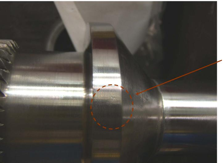
Found damage on probe indicating surface of the 3<sup>rd</sup> stage, impeller end
