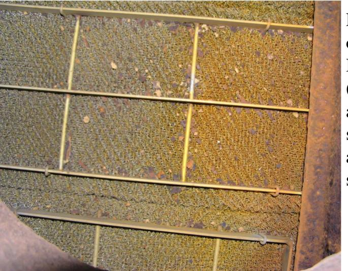
Demister pads on Second Intercooler (between 2<sup>nd</sup> and 3<sup>rd</sup> stage) showing rust and corrosion scale
