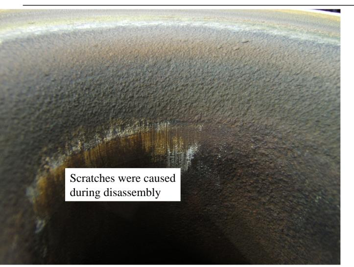
Close up of the 3<sup>rd</sup> stage inlet cone. It shows deposit and rust
