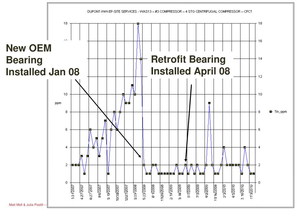
OEM thrust bearing installed between January and April 2008
