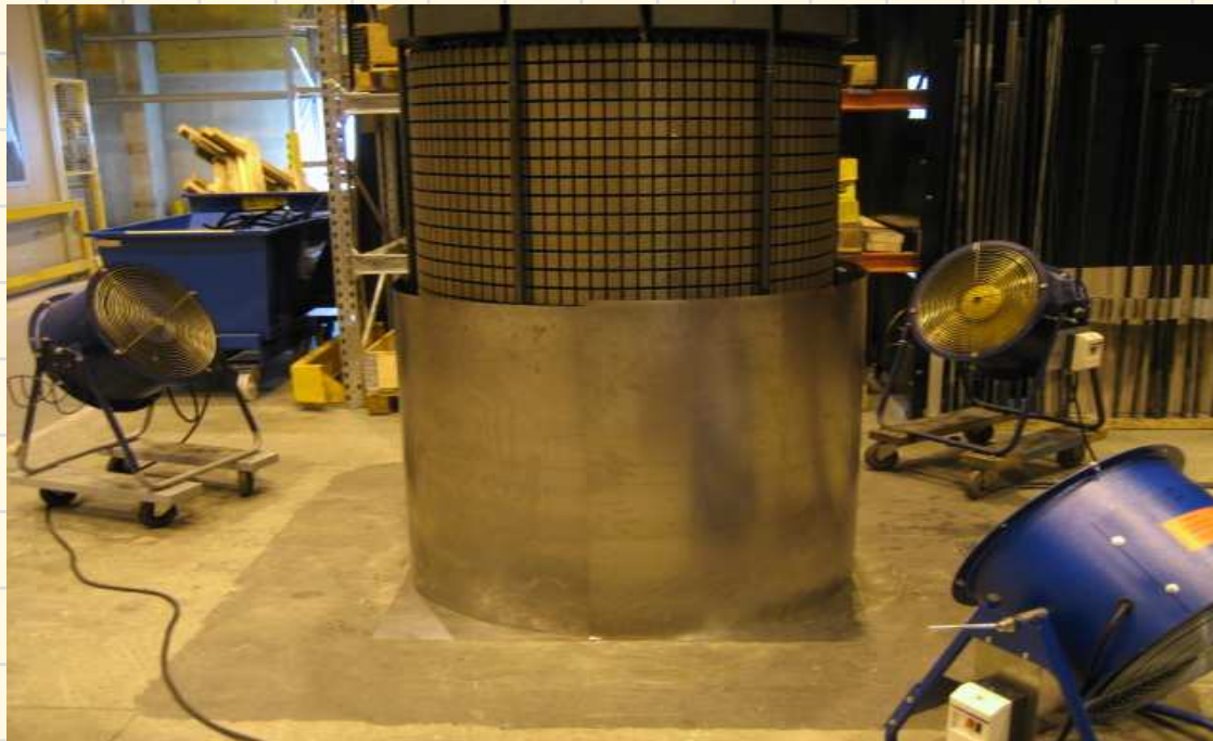
'Insulation' around bottom part of rotor core
