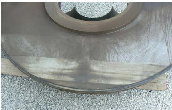
Figure 23. Photograph showing stains on a diaphragm
