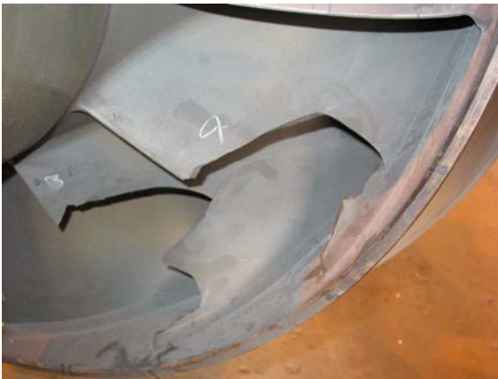
Figure 5. Fourth Impeller released pieces from blade leading edge – June 2007
