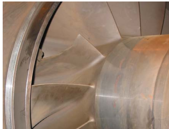
Figure 8. Fourth Impeller released piece at blade leading edge – June 2009
