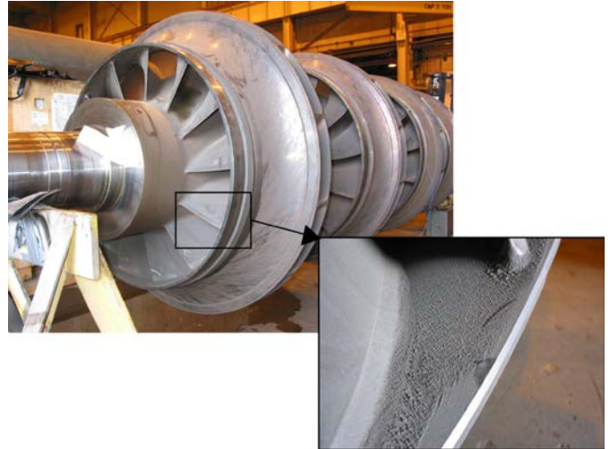
Figure 24. Photograph of the 2007 failed rotor showing swirl patterns on the impellers.
