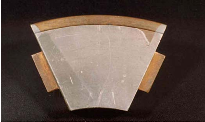
Figure 24 Thrust pad with electrostatic discharge damage
