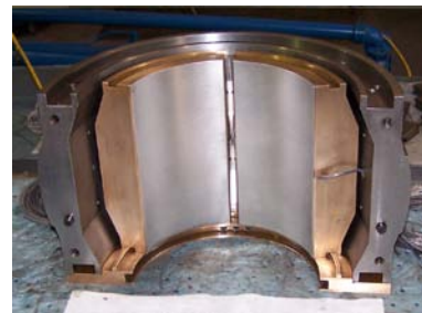
Figure 28 601 bearing after 9 years in operation
