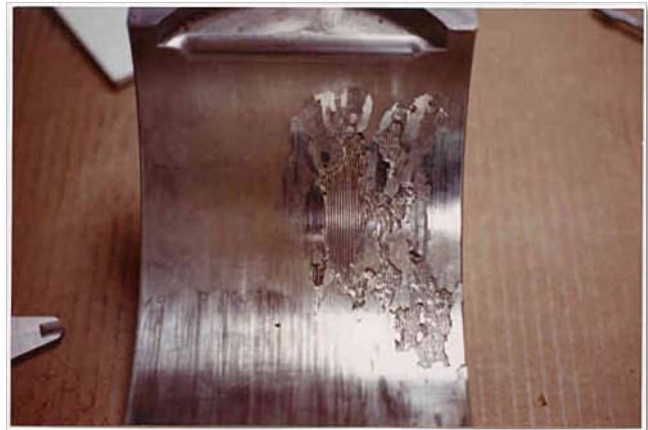
Figure 18 Wiping and fatigue/misalignment
