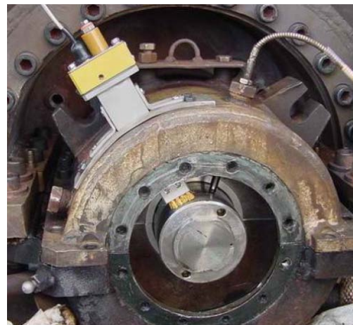
Figure 16- Typical Grounding Brush Installation (Sohre, 2010)
