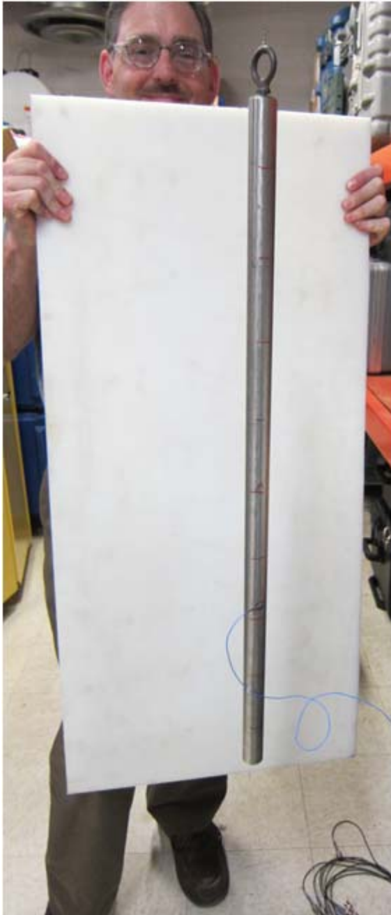
Figure 15. Uniform bar under testing. 28.5” long and 1” in diameter
