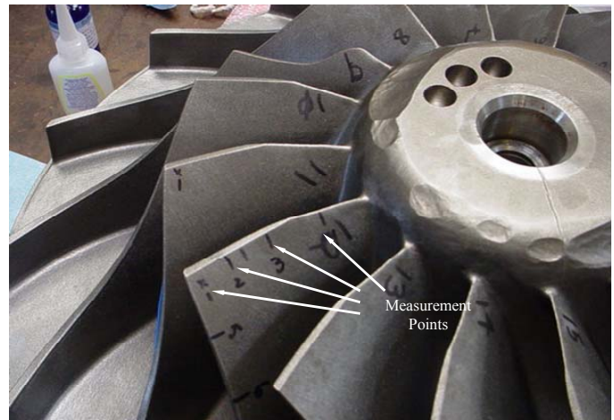
Figure 54. Natural frequencies measurements on the impeller blade.
