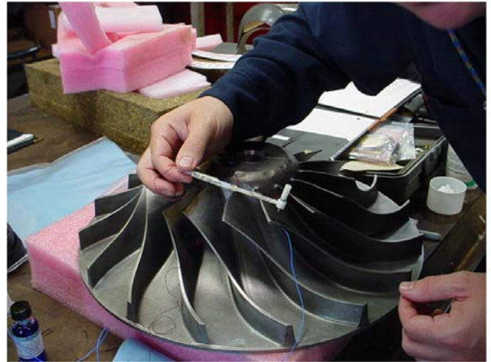
Figure 22. Impact testing of compressor impeller blade
