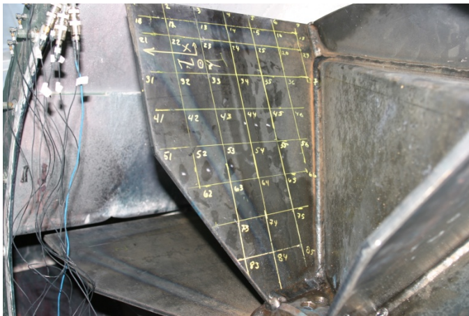
Figure 8. Blade of the shredder fan under testing.
