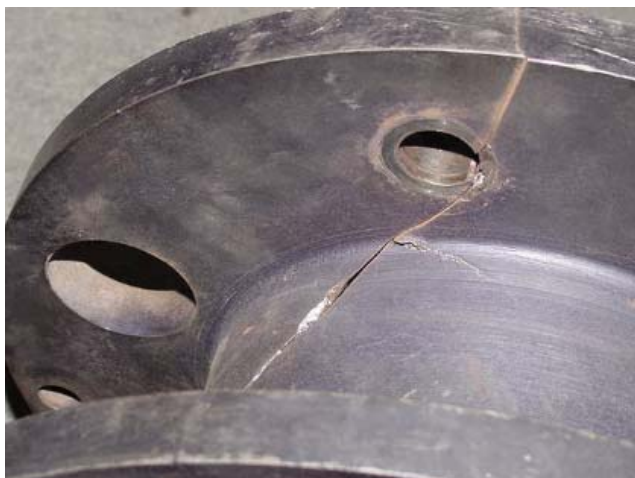
Figure 19. Cracked Coupling Spacer (Bolt Hole).
