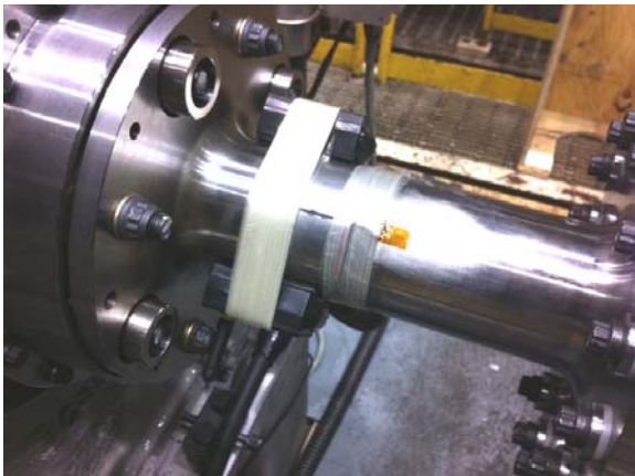
Figure 13. Strain Gage Telemetry System.
