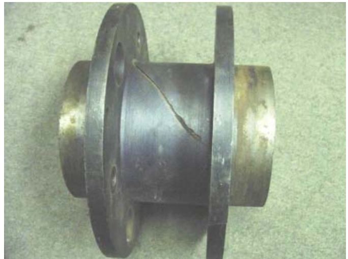
Figure 20. Cracked Coupling (Center Spacer).
