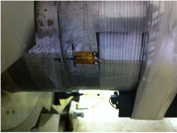
Figure A.3. Close-up View of Chevron Style Strain Gage. Calibration of Strain Gage System
