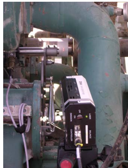
Figure A.9. Laser Aimed at Reflective Tape on Jack Shaft.
