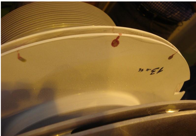
Figure 8. Dye penetrant test at impeller outer diameter.
