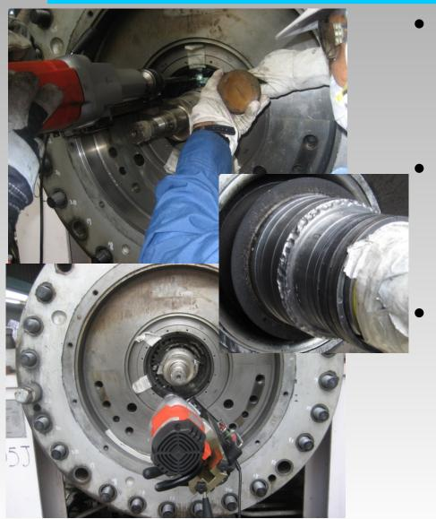
Dry gas seal rotating face fragments (WC) caused damage that impeded compressor disassembly.
