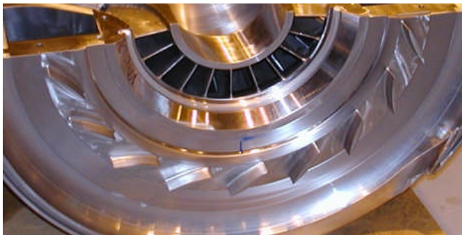
Figure 23. Low solidity diffuser vanes (LSDs)
