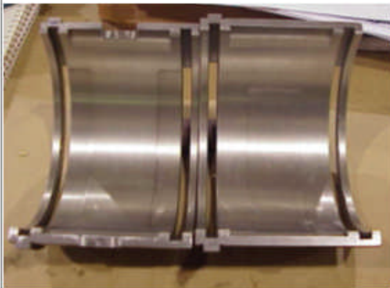
Original Pressure Dam Bearing
