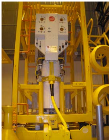
Figure 8. View of one Hybrid Pump module during the structure FAT (Courtesy of Pazflor Project).
