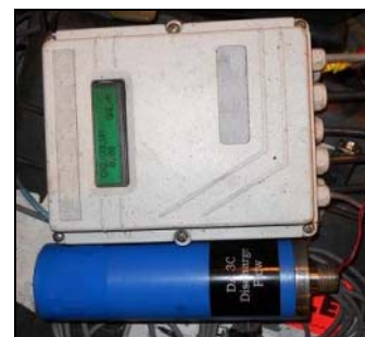
Figure 5. Ultrasonic Flow Meter With Loop Powered Transmitter.
