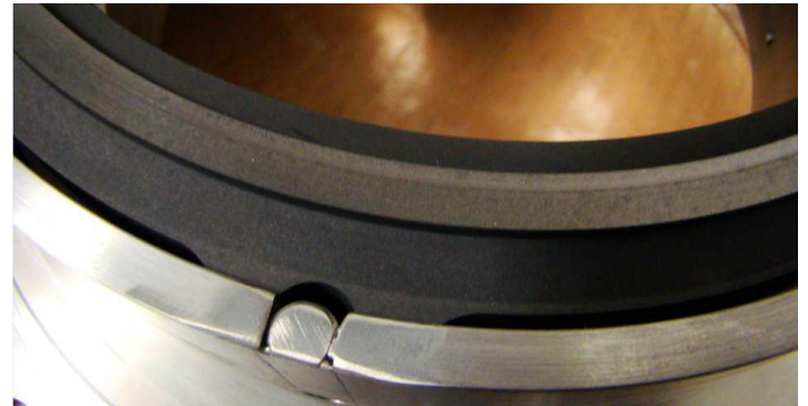
Figure 20. Post-Test Carbon Face
