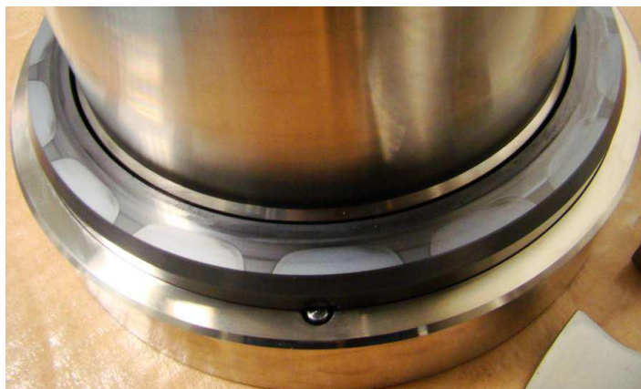
Figure 19. Post-Test 6" Seal Design Wavy SiC Face
