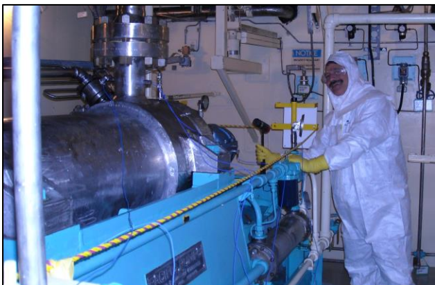
Figure 12. EMA Test at the OBB in the Axial Direction Using a 3 lbm Hammer
