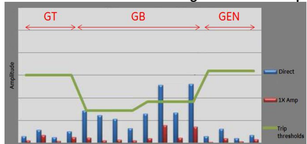
GTG vibrations during MR train start-up
