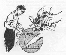
Keep tools clean and free from grease. Select the right chisel for the work being done and check its condition. Wear goggles. Holding a cold chisel between thumb and forefinger with palm up is recommended whenever possible. Keep beveled cutting edge flat against work. Pay strict attention to what you are doing and keep your eye on the cutting edge of tool.
