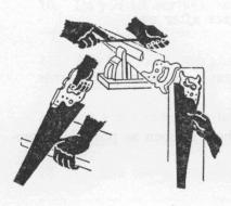
Keep saw sharp, clean, and set teeth properly. Use crosscut saw for cutting across the grain and a rip saw for cutting with the grain. Start a cut with one or two long pulls upward using thumb as guide (see illustration). Then remove hand from danger zone and proceed with long forward cutting strokes. Watch your balance, keep the saw blade in direct line with the cut at 45-60 degree angle. Hang saw up when not in use.
