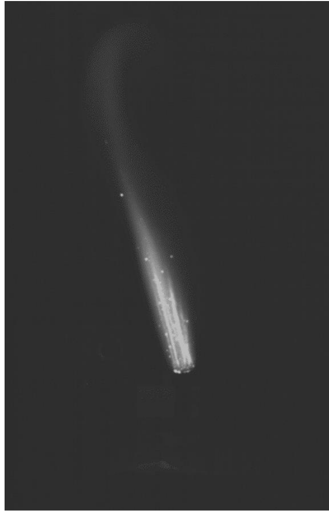
Figure 11. 5% Copper propellant strand burned on vertically adjustable platform. Still image extracted from high speed video taken during burn.
