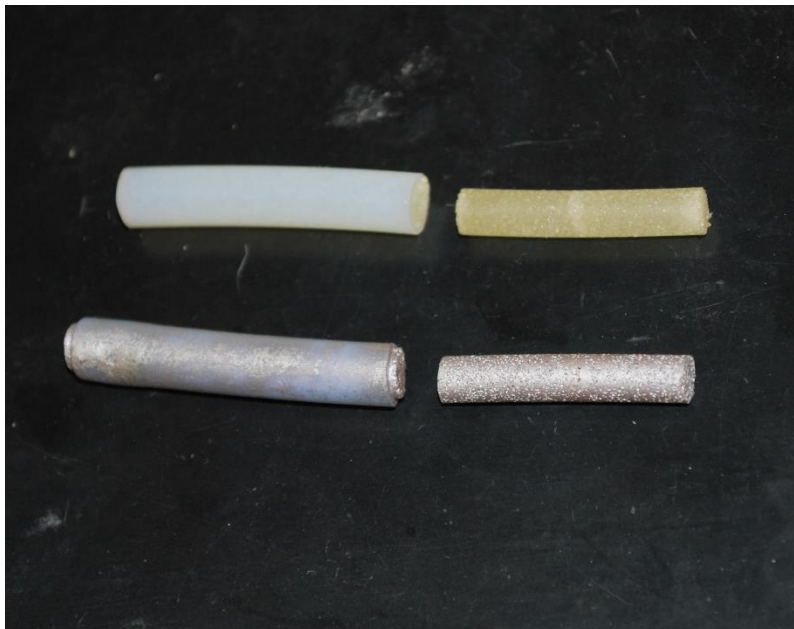
Figure 9. Propellant strands with Teflon tubing (left) and without Teflon tubing (right) [67].
