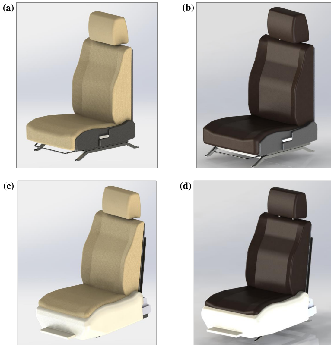
Figure 28: Final modular design of the (a) typical low-end seat, (b) typical high-end seat, (c) accessible low-end seat, and (d) accessible high-end seat
