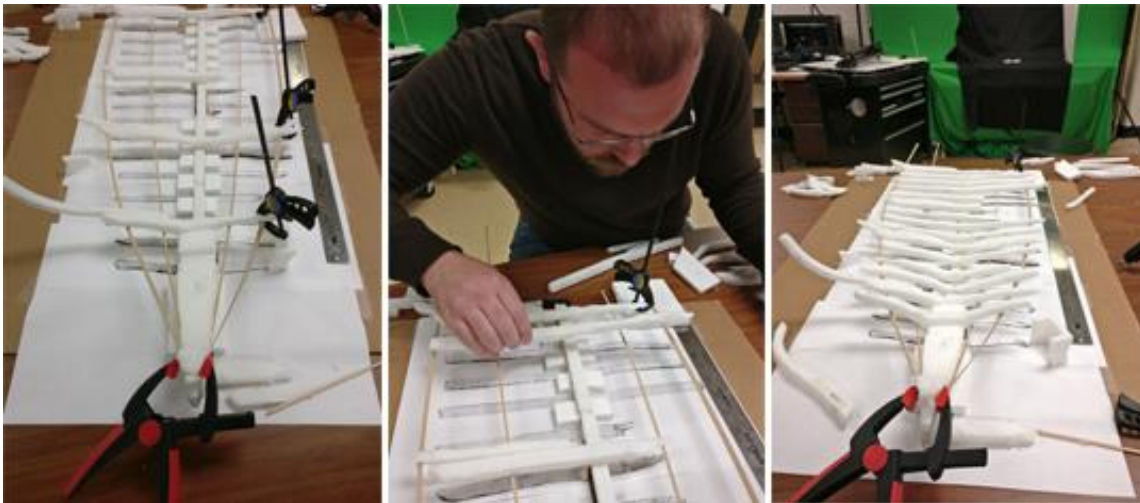
Figure 83: Assembling the physical model. Battens were strung along the master frames and glued in place (left). The author places the remaining floors (center). The model with all floors installed (right). Image by the author.
