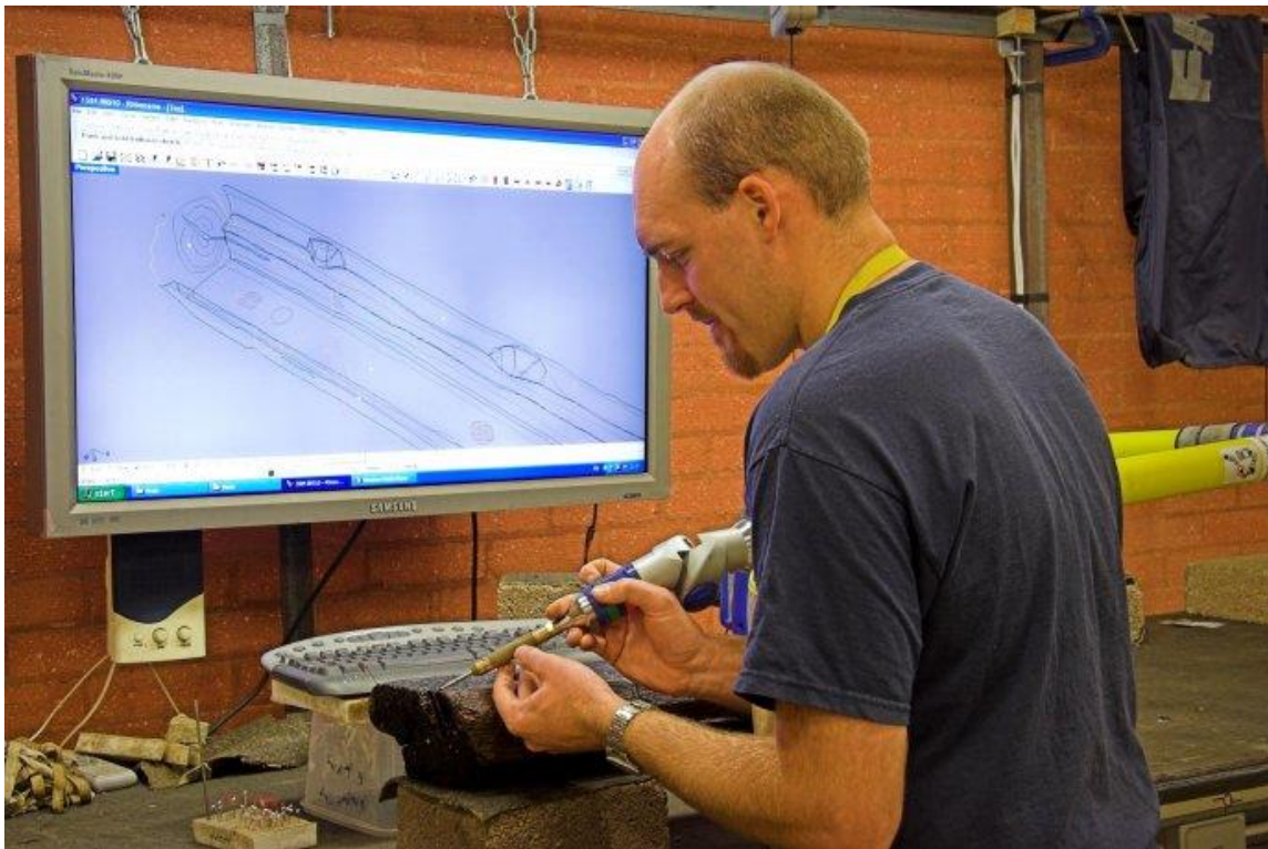
Figure 91: Toby Jones using contact probe digitization to trace a timber from the Newport Ship Project. Reprinted from Friends of the Newport Ship, 2017.
