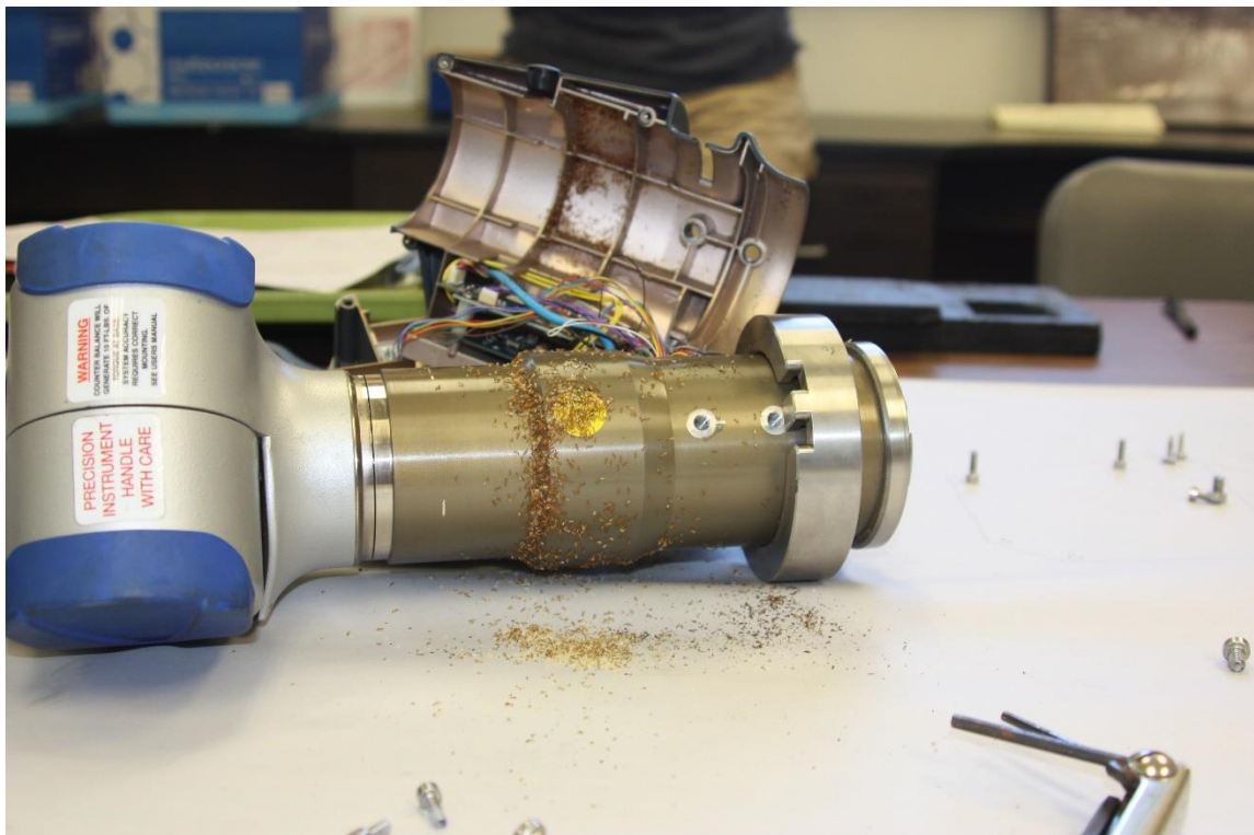
Figure 36: Crazy ant infestation of the FARO Arm circuitry housing. Image by the author.
