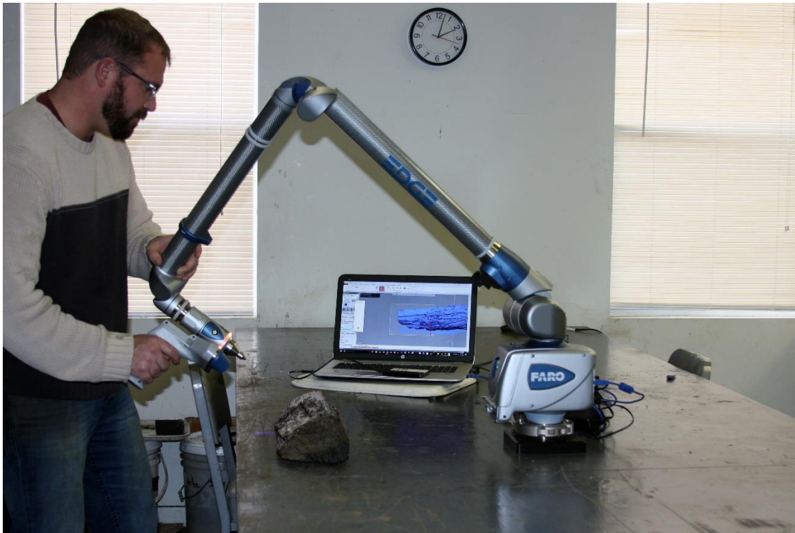
Figure 15: The second scanning arm, the FARO Edge CMM arm with V5 HD LLP, relocated to a new room with a new scanning table in November of 2016. Image by the author.
