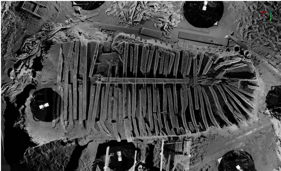
Figure 92: Large-area laser scan of the WTC ship during the excavation. The point cloud is made of six individual scans, as can be seen by the dark circles that represent the blind spots of the scanner. Reprinted from AKRF Inc. 2013.
