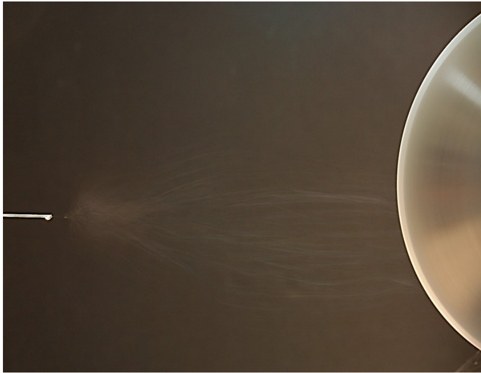
Figure 2.11: Breakup of jet during electrospinning leading to formation of nanofibers
