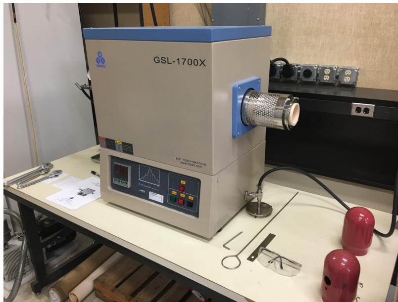
Figure 3.23: Tube furnace used for carbonization
