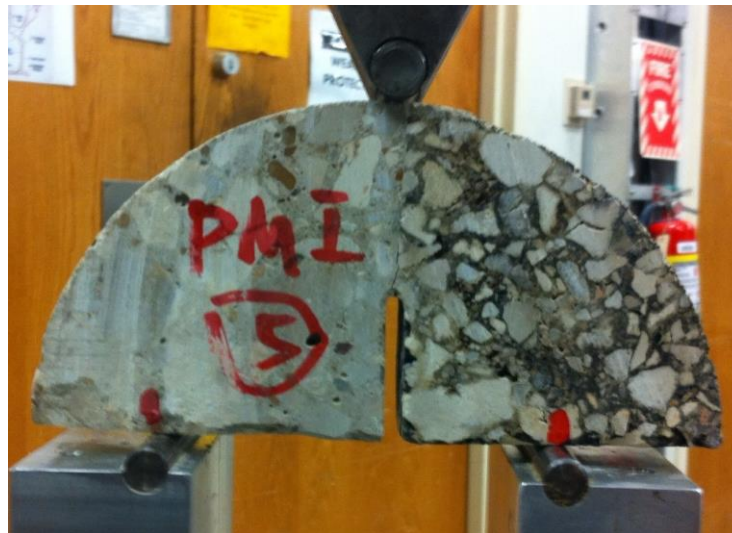
Figure 4-6. Three point bend loading set up for a typical BSCB specimen.
