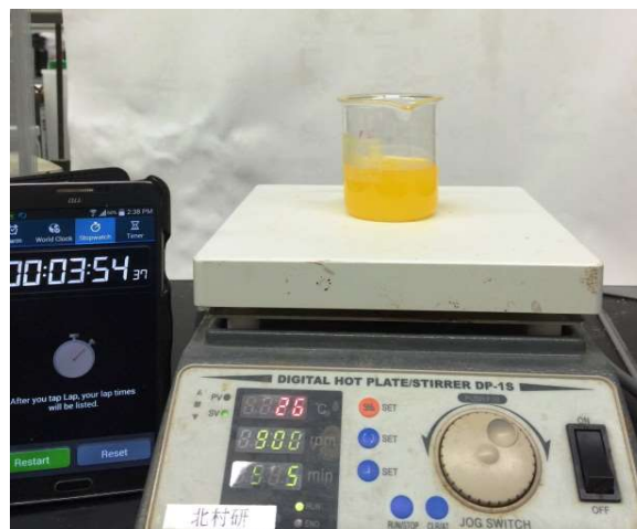
Figure 2-3. Hot plate with magnetic stirrer for determination of rehydration time
