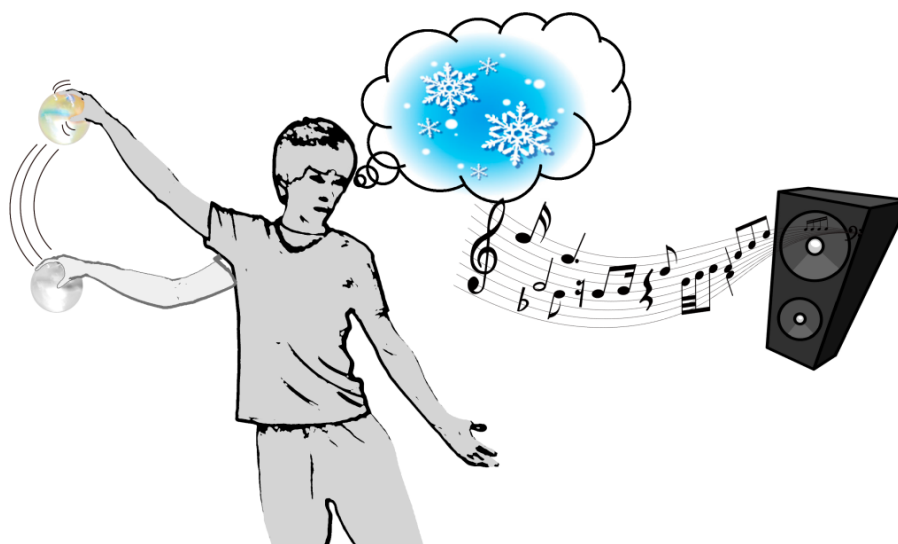
Figure 1. Conceptual diagram for the creative dance support of the proposed grasping-type interface. Motion and grasping force sensed by the interface are presented back to the user in real-time as a variation in musical sound. The sound encourages the user to generate motion continuously and accurately following the imagined trajectory. It also helps the user to conceive imagination for the next motions.
