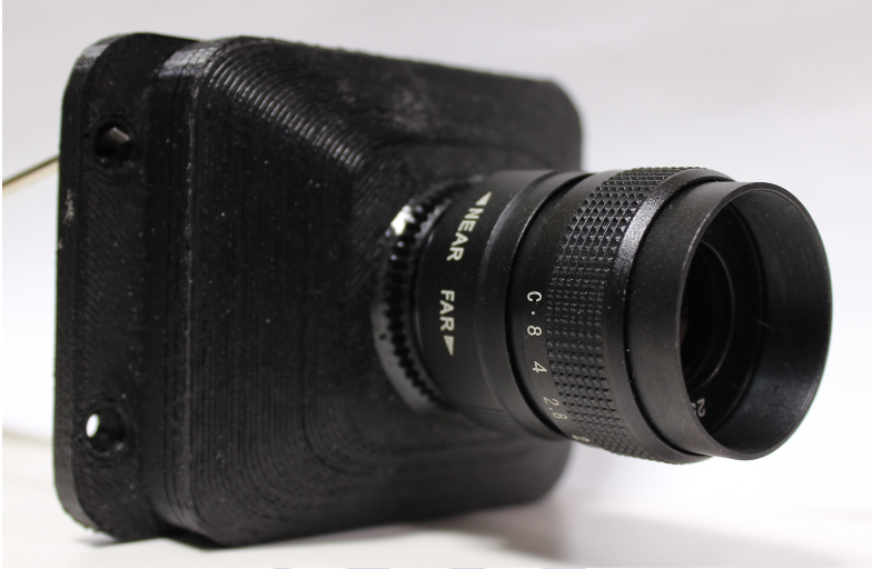
Figure 5.14: Photograph of the 3D printed case and lenses system.
