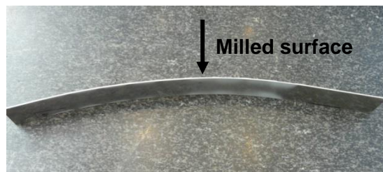
Figure 5. Curvature of the samples milled by AWJ
