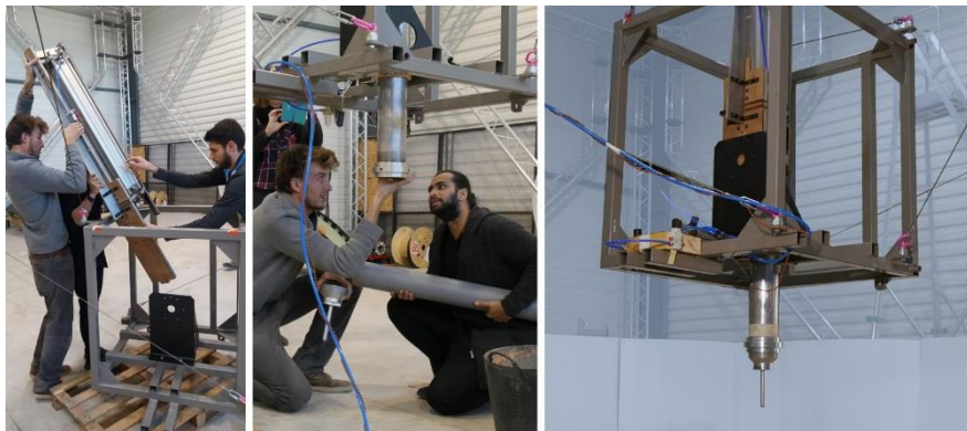
Fig. 2. Assembly of Pylos extruder on Cogiro.
