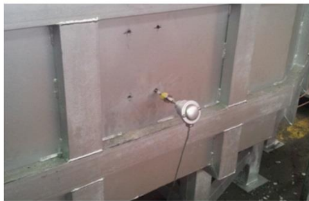
Fig. 3. Measurements performed by means of thermocouples
